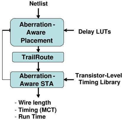
**Figure 6: Aberration-aware timing-driven placement and evaluation flow.**
