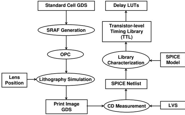
Figure 5: Aberration-aware timing analysis and its flow.
