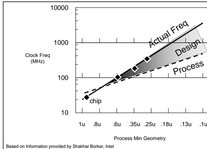
**Figure 3: Pushing Frequency through Process and Design Changes**
