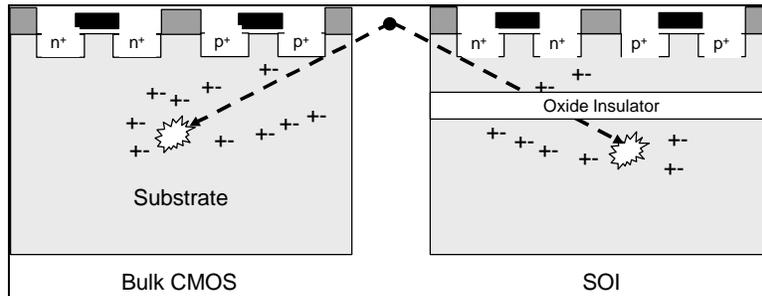
**Figure 26: Soft Errors in CMOS and SOI**
