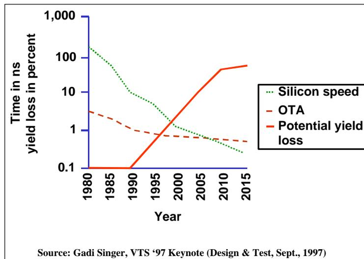
Figure 18: Yield Loss due to Guard Banding
