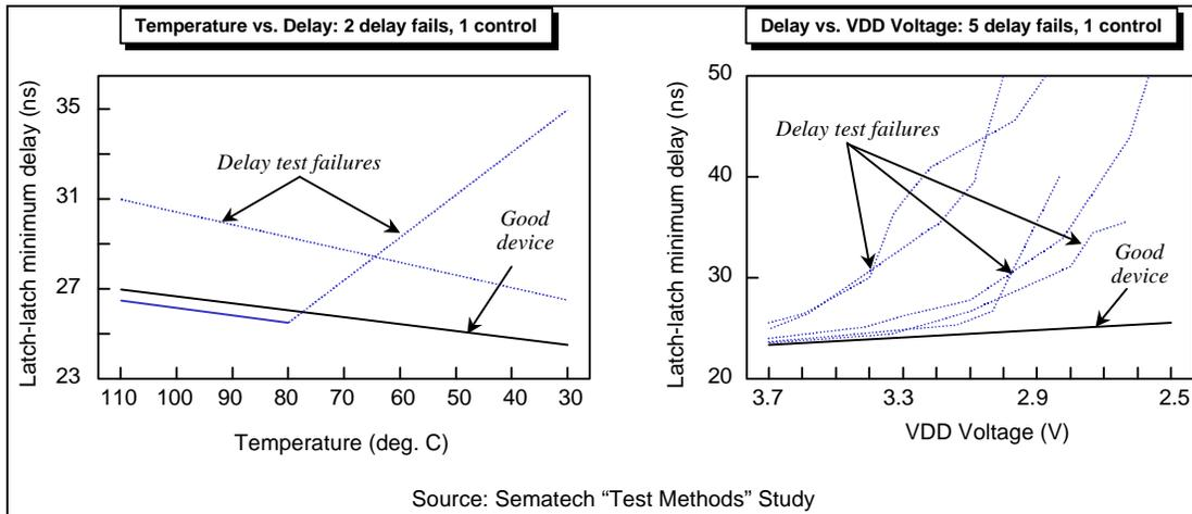
Figure 21: Temperature and Voltage Stress Identifies Faulty Behavior
