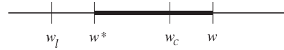
Fig. 1. Relationship between various wire-length quantities. w is a placer's suboptimal wire-length result. w^* is the optimal result. w_l is a lower bound. w_c is a precalculated wire length. w - w^* is the suboptimality gap.
