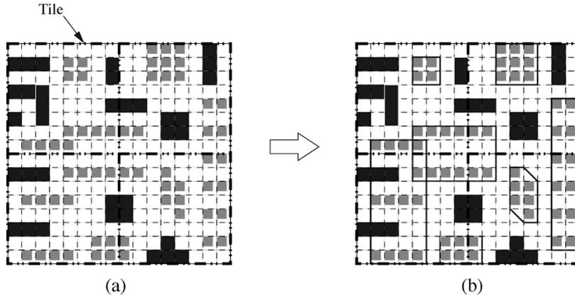
Fig. 4. Example of post-fill compression. (a) Layout divided into four tiles with 61 inserted area fill features. (b) Compressed layout with 61 area fill features using seven OASIS repetitions.
