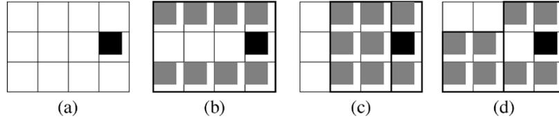
Fig. 8. Comparison of compressible filling using different approaches (Fill requirement = 8). (a) Original tile, the dark solid square shows the occupied original site. (b) Strict Greedy Approach. (c) Greedy Speedup Approach 1. (d) Greedy Speedup Approach 2 ( $K = 2, L = 2$ ).
