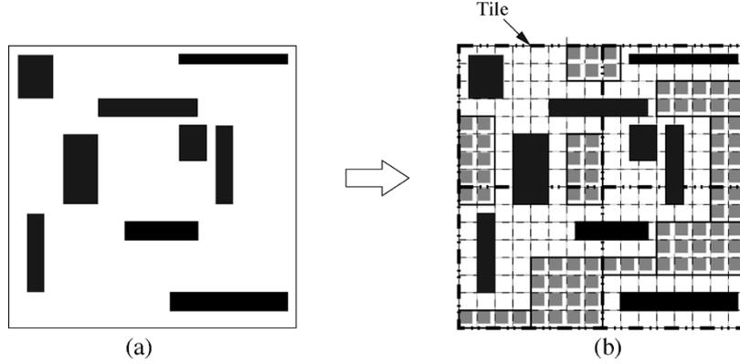
Fig. 3. Example of compressible filling. (a) Original layout. (b) Filled layout with 84 area features in nine AREFs.
