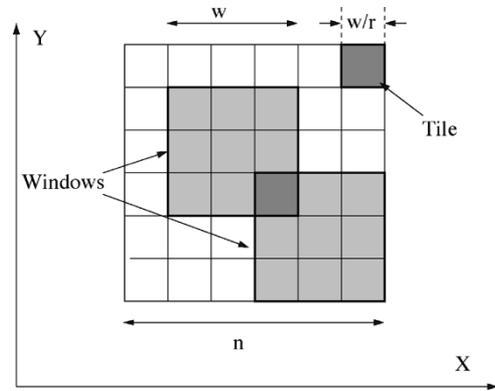
Fig. 1. Fixed  $r$ -dissection regime with parameters  $r = 3$ ,  $w = 3$  and the layout size  $6 \times 6$ . The layout is partitioned by  $r^2 = 9$  distinct  $6 \times 6$  overlapping wrap-around dissections with the phase shift  $w/r = 1$ . There are a total of 36 windows (each tile is a left-bottom tile of a window).
