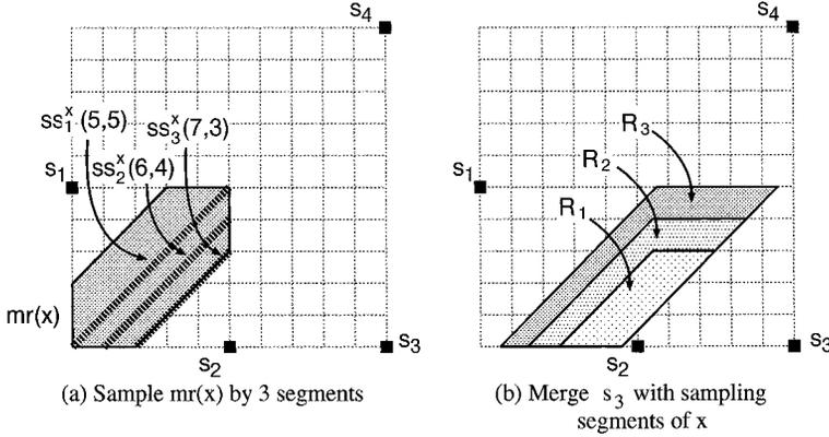
Fig. 12. Interior merging using Manhattan arcs. For the example given in Fig. 11, (a) the merging region  $mr(x)$  is sampled by three Manhattan arcs  $\{ss_1^x, ss_2^x, ss_3^x\}$ . The pair coordinates for each sampling segment denote the max-delay and min-delay of the sampling segment. (b) Merging these sampling segments with sink  $s_3$  produces three merging regions where  $R_i$  is produced by merging  $s_3$  with  $ss_i^x$ .
