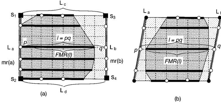
Fig. 10. Example of merging region construction when the joining segments of children merging regions are parallel segments which (a) are vertical or (b) have slopes  $< -1$  or  $> +1$ . (a) presents an example with  $n = 4$  sinks  $s_1, \dots, s_4$ , where there can be up to  $n$  skew turning points on each of  $L_a$  and  $L_b$ . Note that each turning point corresponds to a possible vertex of  $mr(v)$ .
