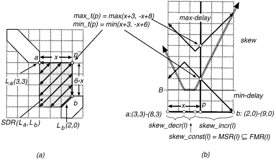
Fig. 6. (a) Merging  $mr(a)$  with  $mr(b)$  using joining segments  $L_a$  and  $L_b$ , respectively. The max-delay and min-delay of  $L_a$  and  $L_b$  are expressed as coordinate pairs. (b) Properties of pathlength delays and skew over the boundary segments  $l = ap + pb$  of  $SDR(L_a, L_b)$ . The first and second coordinate pairs associated with points  $a$  and  $b$  represent (max-delay, min-delay) before and after merging, respectively.
