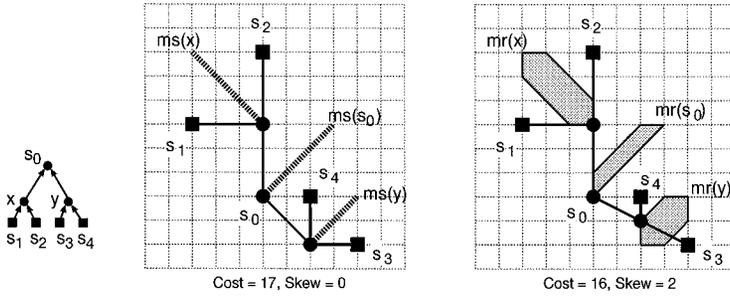
Fig. 1. Comparison of DME zero-skew routing in (b) and BST/DME bounded-skew routing in (c) for the prescribed topology  $G$  in (a). BST/DME lowers the routing cost by allowing non-zero skew bound. Note that in (b) the merging segments are depicted by dashed lines, and in (c) the merging regions are depicted by shaded polygons.
