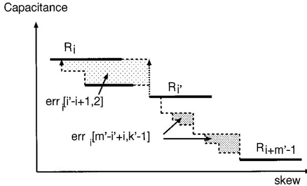
Fig. 25. The lightly shaded region is the area error  $err_i[i' - i + 1, 2]$  for the optimal solution  $S_i[i' - i + 1, 2]$ , i.e., the error incurred when all intermediate regions between  $R_i$  and  $R_{i'}$  are removed. The two darker regions account for the error  $err_{i'}[m' - i' + i, k' - 1]$  of the optimal solution  $S_{i'}[m' - i' + i, k' - 1]$  in case iii of Equation 7.
