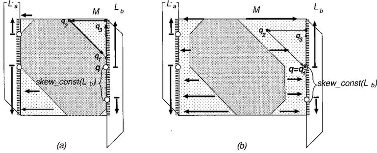
Fig. 22. Proof of the correctness of the BME construction rules for the case where joining segments  $L_a$  and  $L_b$  are vertical, and  $FMR(R) \neq \emptyset$ , where  $R = SDR(L_a, L_b)$ . Arrows indicate the directions of increasing skew/max-delay and decreasing min-delay.
