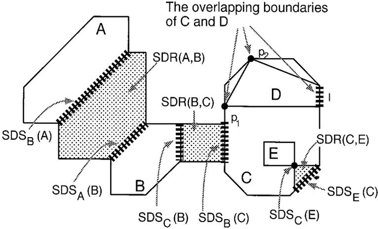
Fig. 5. Examples of Shortest Distance Segments (shown as thick dashed lines or solid dots) and Shortest Distance Regions (shown as dotted regions). Note that the boundaries of polygons *C* and *D* overlap at the two points *p*<sub>1</sub> and *p*<sub>2</sub> and at the line segment *l*. For simplicity, the BME method sets  $SDR(C, D) = l$ .
