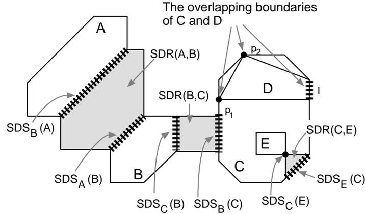
Fig. 5. Examples of Shortest Distance Segments (shown as thick dashed lines or solid dots), and Shortest Distance Regions (shown as dotted regions). Note that the boundaries of polygons  $C$  and  $D$  overlap at the two points  $p_1$  and  $p_2$  and at the line segment  $l$ . For simplicity, the BME method sets  $SDR(C, D) = l$ .
