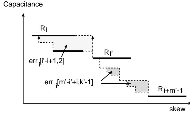
Fig. 25. The lightly shaded region is the area  $err_i[i'-i+1, 2]$  for the optimal solution  $S_i[i'-i+1, 2]$ , i.e., the error incurred when all intermediate regions between  $R_i$  and  $R_{i'}$  are removed. The two darker regions account for the error  $err_{i'}[m'-i'+i, k'-1]$  of the optimal solution  $S_{i'}[m'-i'+i, k'-1]$  in case (iii) of Eqn. (7).
