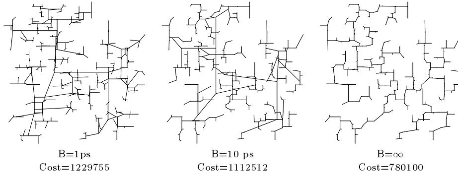
Fig. 20. Layout of BME routing solutions for benchmark r1 with skew bound  $B = 1, 10,$  and  $\infty$  ps.
