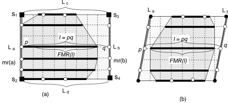
Fig. 10. Example of merging region construction when the joining segments of children merging regions are parallel segments which (a) are vertical or (b) have slopes  $< -1$  or  $> +1$ . In (a) is an example with  $n = 4$  sinks  $s_1, \dots, s_4$ , where there can be up to  $n$  skew turning points on each of  $L_a$  and  $L_b$ . Note that each turning point corresponds to a possible vertex of  $mr(v)$ .
