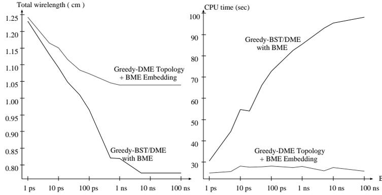
Fig. 19. Comparisons of (a) total wirelength and (b) run-times between topologies produced by Greedy-BST/DME and Greedy-DME for various skew bounds from  $1\text{ ps}$  to  $100\text{ ns}$
