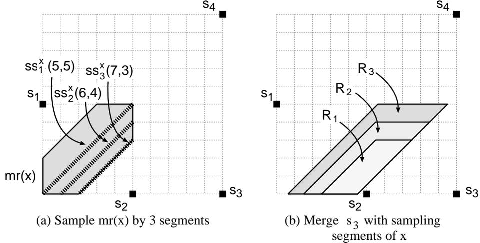
Fig. 12. Interior merging using Manhattan arcs. For the example given in Fig. 11, (a) the merging region  $mr(x)$  is sampled by three Manhattan arcs  $\{ss_1^x, ss_2^x, ss_3^x\}$ . The pair coordinates for each sampling segment denote the max-delay and min-delay of the sampling segment. (b) Merging these sampling segments with sink  $s_3$  produces three merging regions where  $R_i$  is produced by merging  $s_3$  with  $ss_i^x$ .
