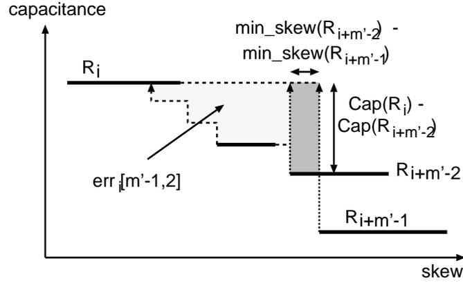
Fig. 24. The lightly shaded region is the area  $err_i[m'-1, k'=2]$  for the optimal solution  $S_i[m'-1, k'=2]$ , i.e., the error incurred when all intermediate regions between  $R_i$  and  $R_{i+m'-2}$  are removed. The darker region is the additional error incurred when region  $R_{i+m'-2}$  is also removed. It is the skew-capacitance product term in case (ii) of Eqn. (7).
