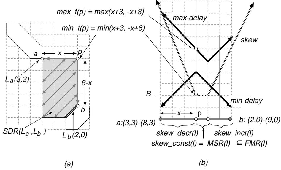
Fig. 6. (a) Merging  $mr(a)$  with  $mr(b)$  using joining segments  $L_a$  and  $L_b$ , respectively. The max-delay and min-delay of  $L_a$  and  $L_b$  are expressed as coordinate pairs. (b) Properties of pathlength delays and skew over the boundary segments  $l = \overline{ap} + \overline{pb}$  of  $SDR(L_a, L_b)$ . The first and second coordinate pairs associated with points  $a$  and  $b$  represent (max-delay, min-delay) before and after merging, respectively.
