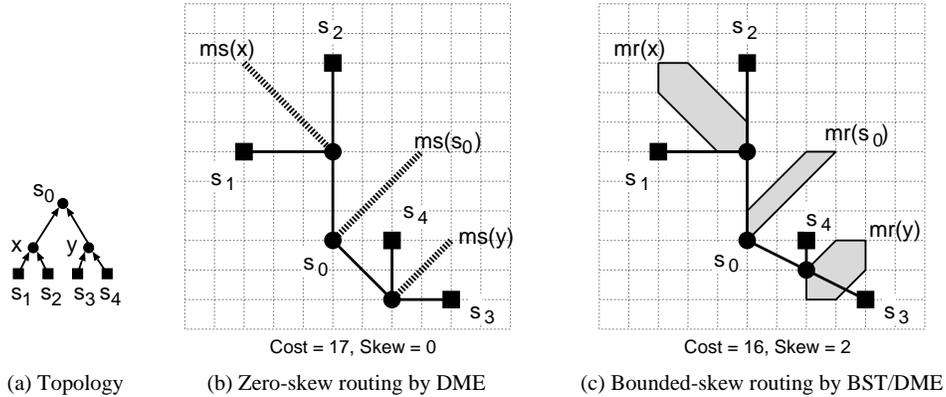
Fig. 1. Comparison of DME zero-skew routing in (b) and BST/DME bounded-skew routing in (c) for the prescribed topology  $G$  in (a). BST/DME lowers the routing cost by allowing non-zero skew bound. Note that in (b) the merging segments are depicted by dashed lines, and in (c) the merging regions are depicted by shaded polygons.
