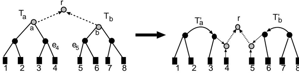
Fig. 15. An example showing that given skew bound  $B \gg 0$ , changing the subtree topology before merging will reduce the merging cost.
