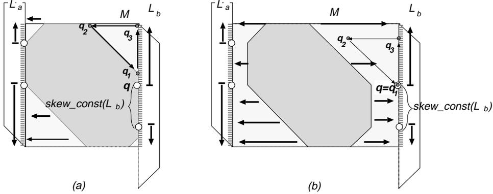
Fig. 22. Proof of the correctness of the BME construction rules for the case where joining segments  $L_a$  and  $L_b$  are vertical, and  $FMR(R) \neq \emptyset$ , where  $R = SDR(L_a, L_b)$ . Arrows indicate the directions of increasing skew/max-delay and decreasing min-delay.
