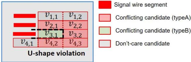
Fig. 8. Illustration of a U-shape block mask rule violation.
