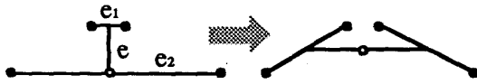
Figure 3: Example of flipping an H as to minimize clock skew: the clock tree on the left has no zero-skew balance point along the middle segment of the H, while the clock tree on the right does.
