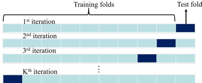
Fig. 7: Diagram of the K-fold cross-validation.
