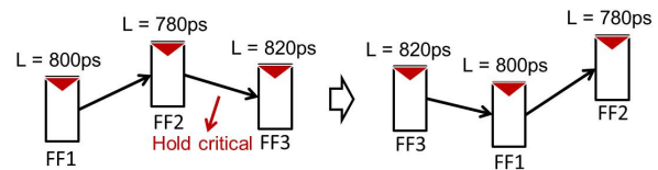
Figure 1: Illustration of skew-aware scan ordering that removes hold violation. L is clock latency.
