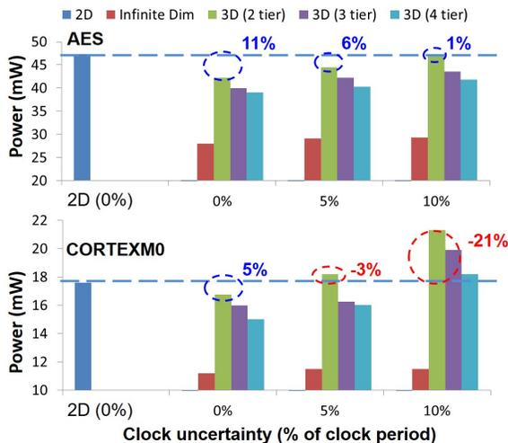
Fig. 3. The impact of larger clock skew (due to complexity of 3D CTS as well as inter-tier variation) on 3D power benefits.
