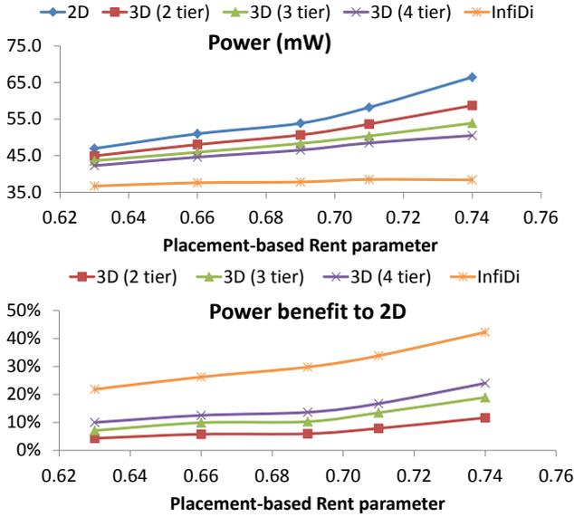
Fig. 4. Power and power benefits versus Rent parameters for the 2D and the 3D implementations with different tiers.
