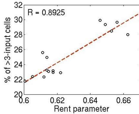
Fig. 6. Correlation between incidence of cells with >3 inputs vs. Rent parameter.
