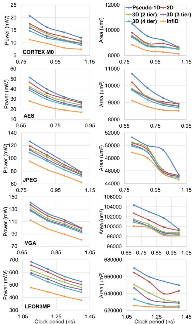
Fig. 2. Design power and total cell area evaluated across various implementation dimensions.
