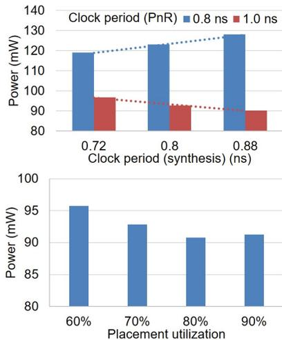
Fig. 1. Design power with (i) varying synthesis clock period, and (ii) placement utilization. Design: JPEG. Technology: 28FDSOI.
