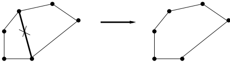
Figure 8. Deleting all common edges (in this case, only one) results in a merged face.
