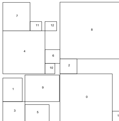
Figure 7. The reticle floorplan for testcase “Ind 2”.
