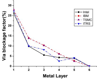
Figure 1: Via blockage in 130nm technology
