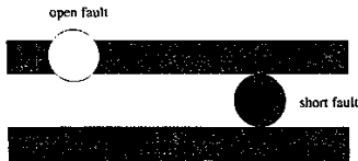
Figure 1: An open fault is formed due to loss of mass; a short fault is formed due to augmentation of mass.
