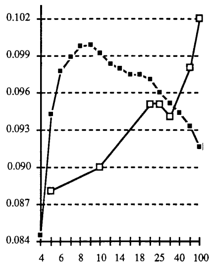
Figure 5: Comparison between Bubble-MRST (square dots) and the optimal MST-based (S-MST) method of Ho, Vijayan and Wong (boxes). The horizontal axis gives net size, and the vertical axis gives improvement over MST cost averaged over 10000 random instances.
