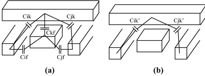
Fig. 1. Graph-based capacitance reduction. (a) Initially, capacitances between all metals are computed. (b) Capacitances to fills eliminated one by one.
