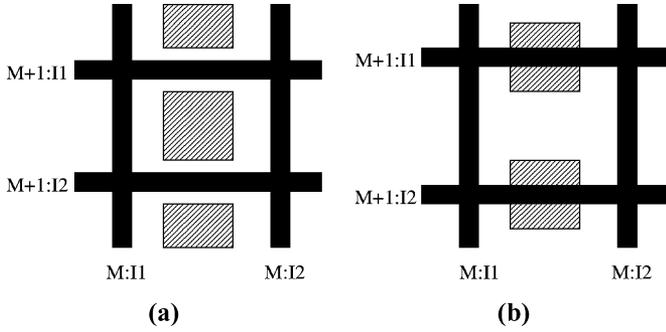
Fig. 7. Interlayer coupling for neighboring layers. (a) Fills on layer  $M$  (vertical) intersect minimally with interconnects on layers  $M-1$  and  $M+1$  (horizontal, overlapping). (b) Fills on layer  $M$  shifted and intersect maximally with interconnects on layers  $M-1$  and  $M+1$ .
