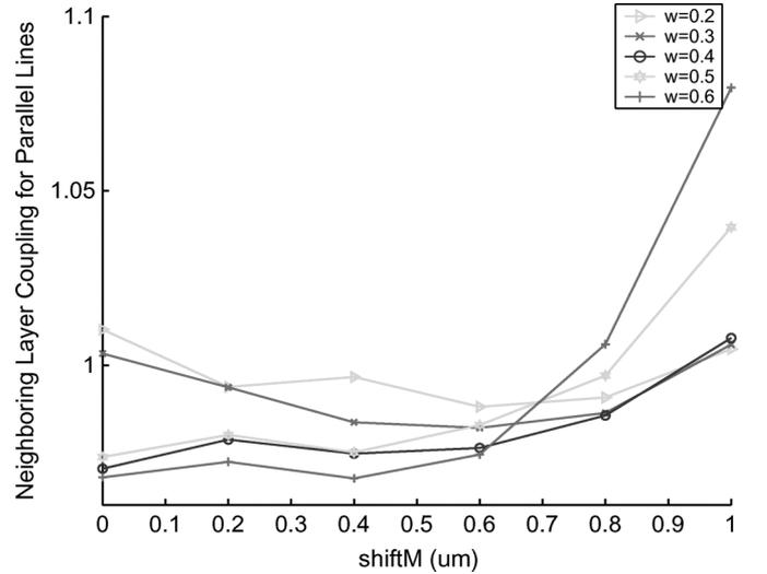
Fig. 17. Neighboring-layer parallel line coupling dependency on amount of  $M$  layer shift for various metal widths.
