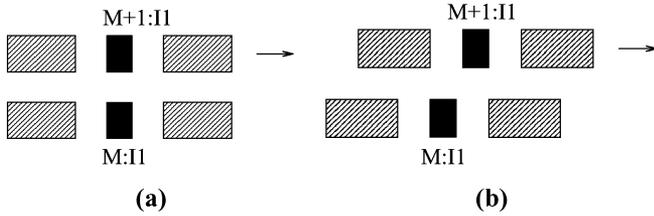
Fig. 8. Interlayer coupling for parallel neighboring lines. (a) Layer  $M$  and  $M+1$  interconnects intersect. (b) Layer  $M+1$  shifted.
