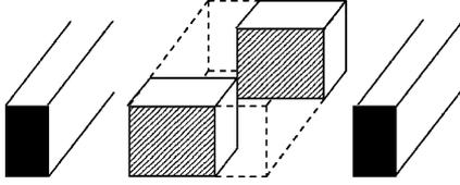
Fig. 4. Fill merging methodology. Fills are patterned and interconnects are represented by dark lines. Dashed box shows merged fill, resulting from convex hull of intralayer neighboring fills.
