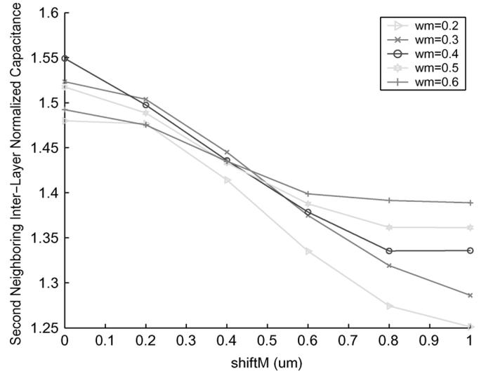
Fig. 18. Fill shift dependency of second neighboring-layer coupling for different metal widths.
