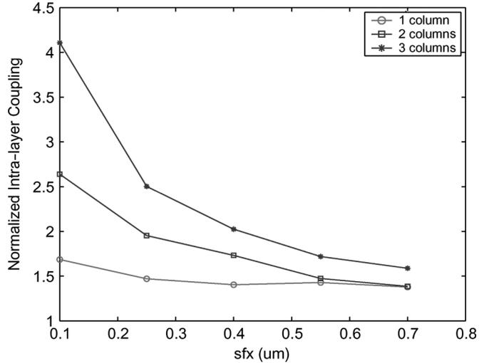
Fig. 15. Fill spacing dependency of intralayer coupling for different number of fill columns.
