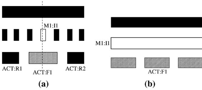
Fig. 11. Active fill DOE simulation structure. (a) Side view. (b) Side view along dashed line. Active regions fills are shown as patterned. Control interconnect is light colored.
