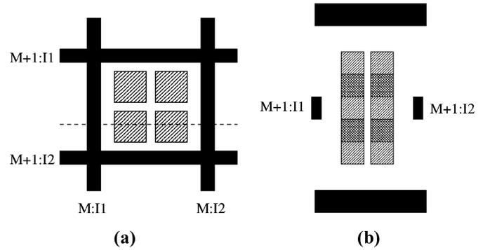
Fig. 10. Via fill DOE simulation structure. (a) Top view. CMP fills laid out in traditional pattern shown.  $M+1$  and  $M-1$  layer interconnects are overlapping. Top and bottom ground planes not shown. (b) Side view along dashed line. Via fills connecting CMP fills on neighboring layers indicated by darker patterns.
