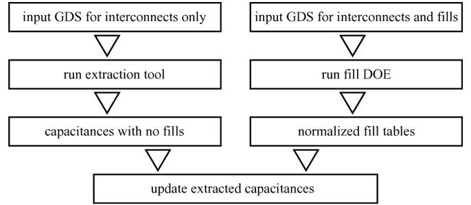
Fig. 5. Proposed flow to incorporate floating fill impact.
