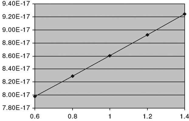
Fig. 13. CMP-induced height impact on coupling capacitance shows linear change. Nominal coupling capacitance in Farads as a function of normalized metal height shown.
