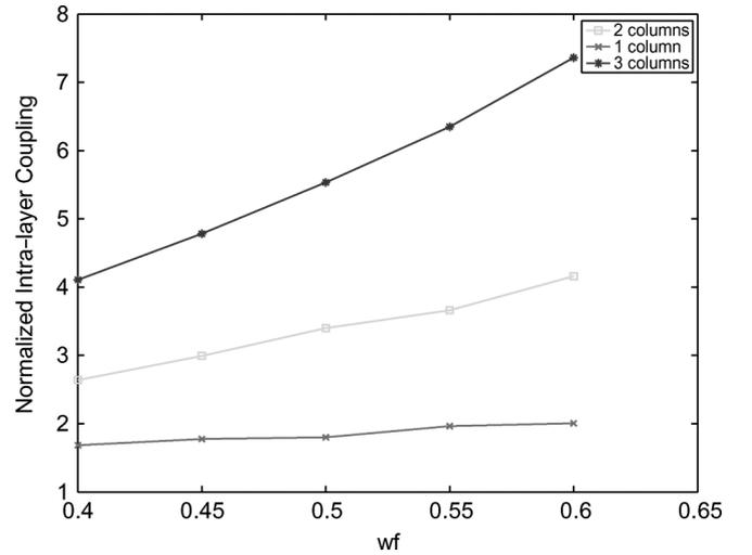
Fig. 14. Fill width dependency of intralayer coupling for different number of fill columns.
