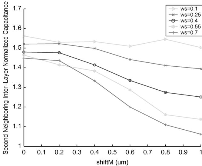
Fig. 19. Fill shift dependency of second neighboring-layer coupling for different fill-to-fill spacings.
