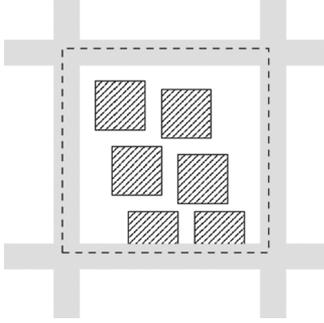
Fig. 6. Basic DOE structure. Structure consists of five layers. Top and bottom are ground planes. Three layers consist of parallel interconnects orthogonal to others across each layer. Structure enables observation of intralayer and first and second neighboring layer couplings in one simulation. Fills are patterned and interconnects are represented by solid gray lines.
