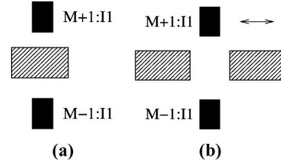
Fig. 9. Interlayer coupling for second neighboring layers. (a) Fills on layer  $M$  intersect maximally with interconnects on layers  $M-1$  and  $M+1$ . (b) Fills on layer  $M$  shifted and intersect minimally with interconnects on layers  $M-1$  and  $M+1$ .
