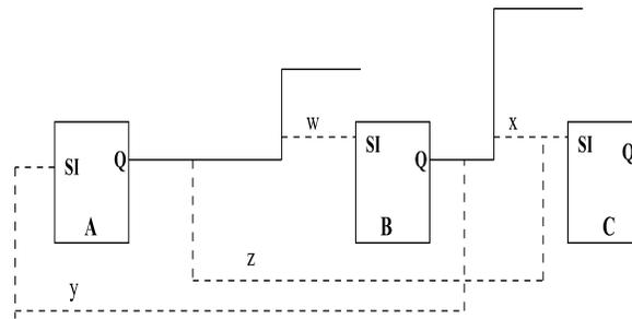
Fig. 2. An example showing the highly asymmetric and nonmetric nature of the ATSP when doing incremental scaninsertion.
