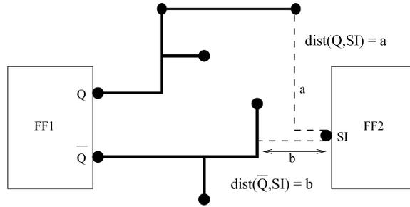
Fig. 3. Pin-to-Net distance measurement for routing-driven scan ordering.
