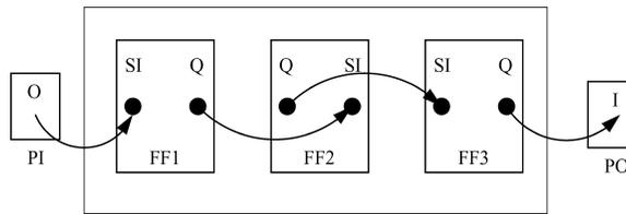
Fig. 1. Example of a scan chain with three scan registers  $FF1$ ,  $FF2$ , and  $FF3$ . In each sequential cell,  $SI$  and  $Q$  denote the scan-in pin and scan-out pin.  $PI$  is the primary input pad, and  $PO$  is the primary output pad.
