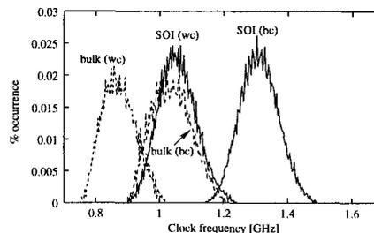
Figure 4: Parameter sensitivity for bulk Si and SOI device models.
