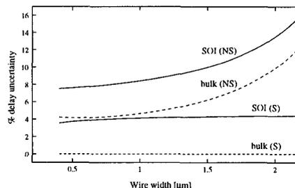
Figure 5: Delay uncertainty for staggered (S) and non-staggered (NS) repeater topologies using bulk and SOI. Results are for a 1.5cm global wire with four 100X repeaters.
