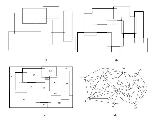
Figure 1: (a) A global floorplanning result (rectangles); (b) the contour (defining whitespace); (c) whitespace and overlap within the layout region; and (d) the corresponding graph.
